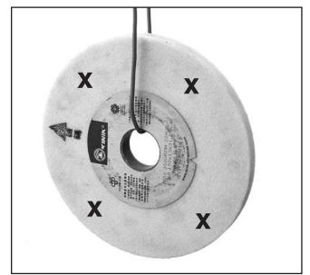
Figure 29. Ring test setup.
